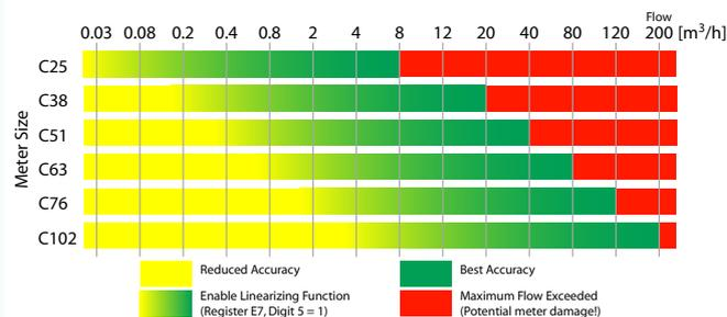
When selecting the meter size, use the diagram to the left and observe the following guidelines:
